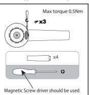
B. Assemble the cover plate to the motor housing with 2 x screws provided. Max. torque to 0.5 Nm.
